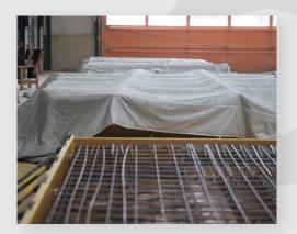
We clearly see the advantages of using thermal concrete duvets, as opposed to PE foil. The heat for the curing process is kept more stable and condensate is not a problem.
